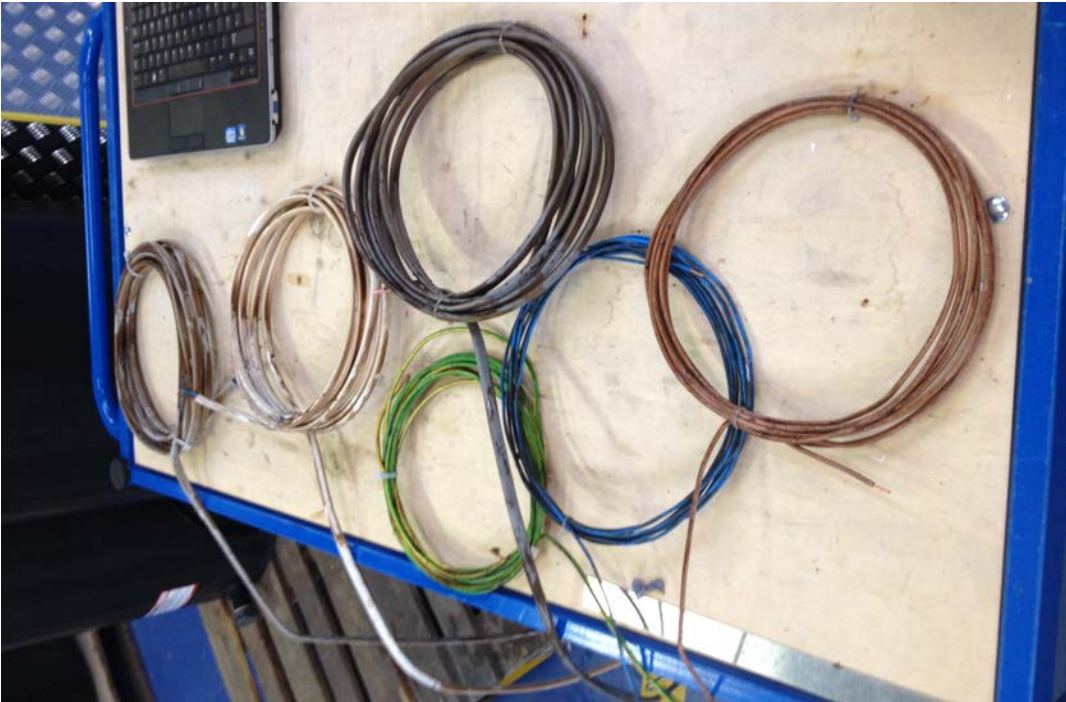
Figure 3: Condition of the cables after Protocol 2 - Penetration.
