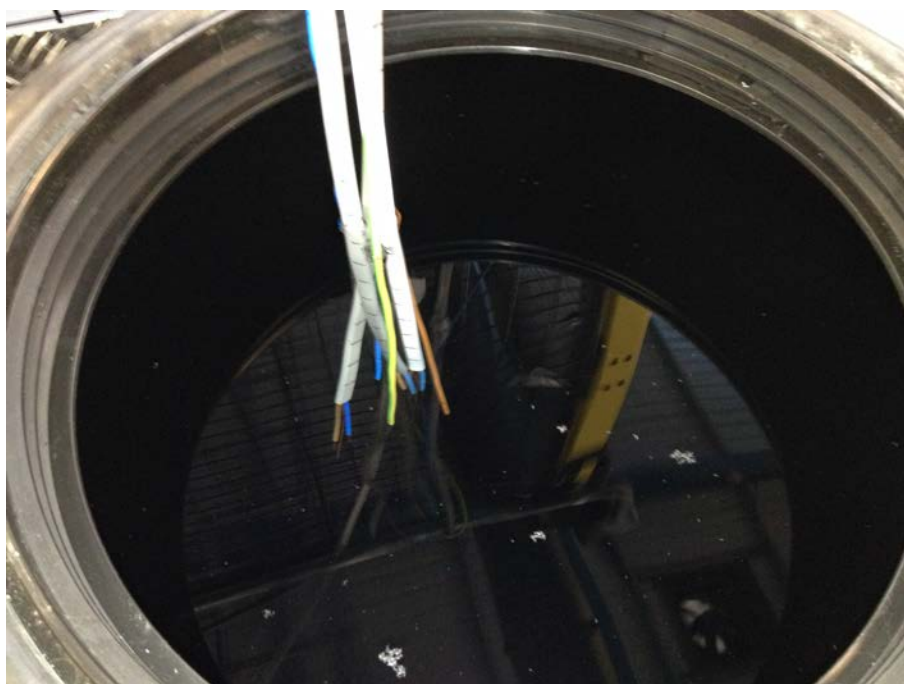
Figure 2: Arrangement of cable ends dipped into the liquid (Protocol 1 – Wicking).
