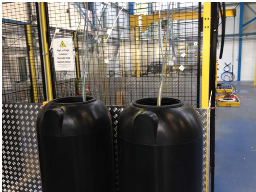
Figure 1: Arrangement of tanks and suspension of cables.
